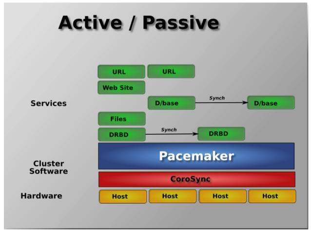
Pacemaker also supports multiple nodes in a shared-failover design, reducing hardware costs by allowing several active/passive clusters to be combined and share a common backup node.
