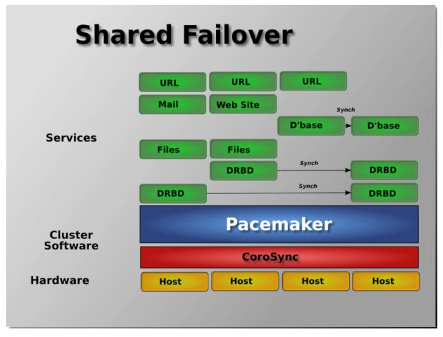
When shared storage is available, every node can potentially be used for failover. Pacemaker can even run multiple copies of services to spread out the workload. This is sometimes called N-to-N redundancy.
